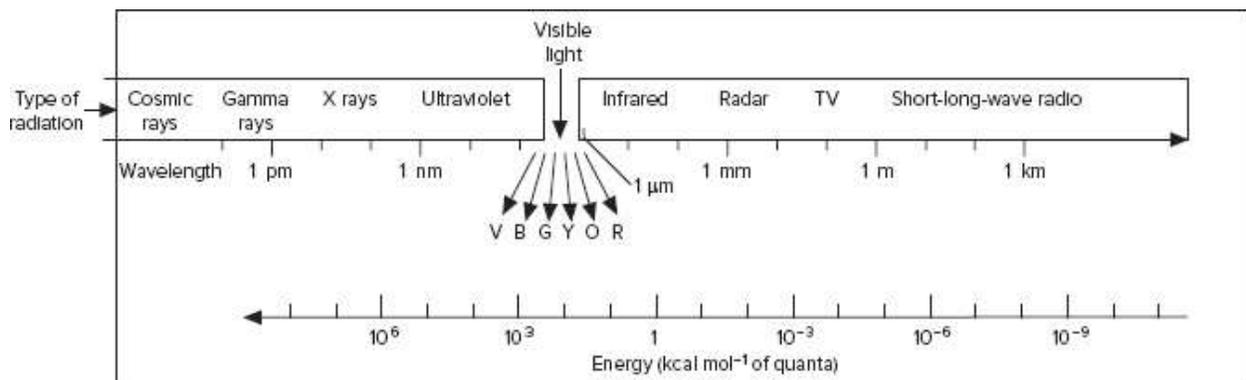
**FIGURE 17.16 The spectrum of electromagnetic radiation.** Between extremely short cosmic rays and long radio waves lies a narrow band of “visible light,” to which human eyes are normally sensitive. Wavelength increases to the right. Energy within the electromagnetic
