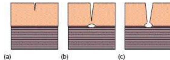
**FIGURE 4.38 Fracture propagation.** (a) Failure of a structure begins with the appearance of a microfracture that spreads rapidly. (b) In composite materials, such as bone, the advancing fracture is preceded by stress waves that may cause the concentrated force to spread at the boundary between the composite materials, where they give slightly. (c) As the fracture line meets this boundary, its sharp tip is blunted and its progress curtailed.
