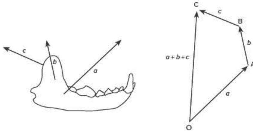
**FIGURE A.2 Addition of multiple vectors.** Several vectors,  $a$ ,  $b$ ,  $c$ , acting simultaneously on the carnivore lower jaw can be added graphically (right) to determine the single resultant,  $a + b + c$ , of their collective action (left).
