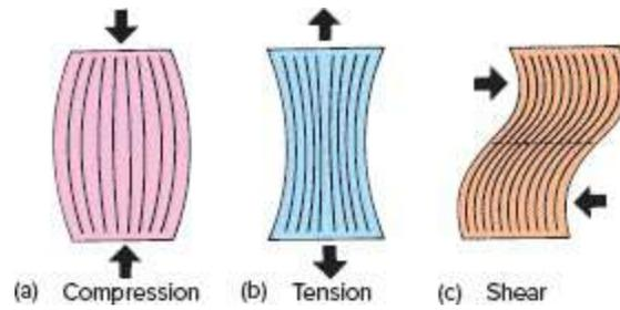
**FIGURE 4.34 Direction of force application.** The susceptibility of a material to breaking depends on the direction in which the force is applied (arrows). Most materials withstand compression best (a) and are weaker when placed in tension (b) or shear (c).
