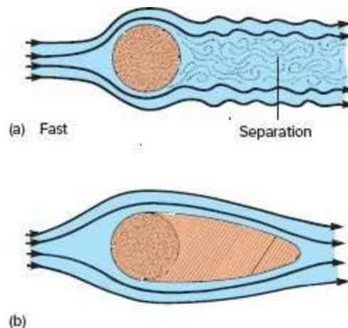
**FIGURE 4.29 Streamlining.** (a) Particles in the boundary layer are unable to make the sharp change in direction and velocity to negotiate the turn around the cylinder-shaped object, and flow separation occurs behind the object. (b) Extension and tapering of the object into the area of disturbance help prevent separation and result in a streamline shape.
