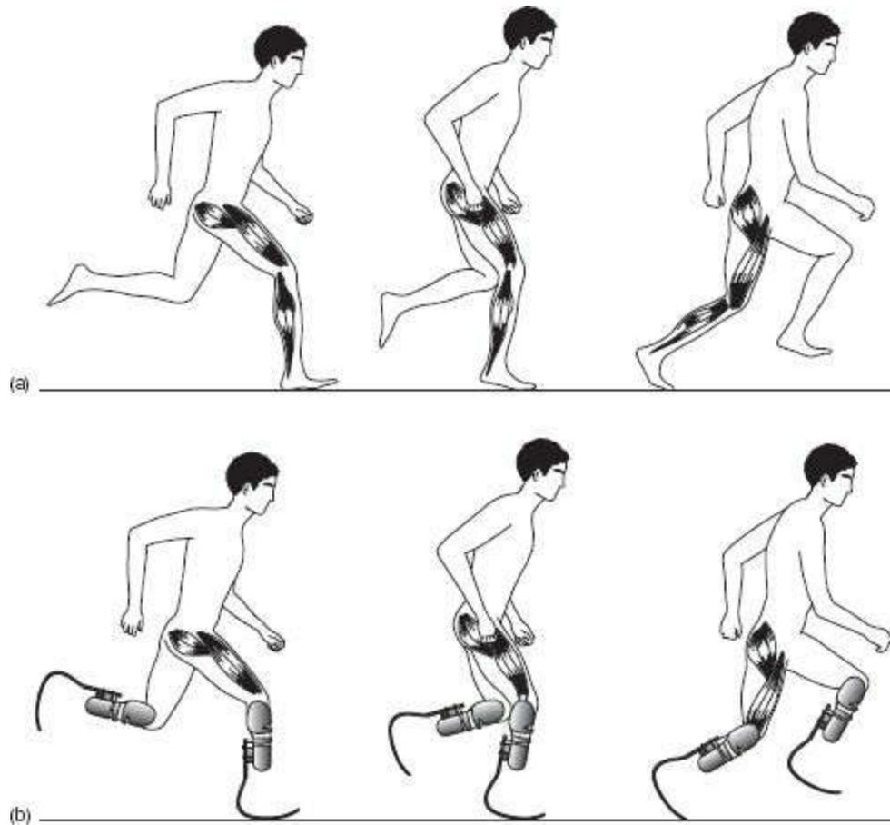
**BOX FIGURE 1 Running blades.** (a) During a normal running gait, the lower leg stores mechanical energy on footfall and elastically returns it at foot push-off. Active muscle contraction adds to this elastically returned force. (b) The curved blade acts mechanically in a similar way, storing mechanical energy on contact and elastically returning it at push-off.
